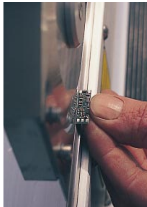
High value circuitry with intermittent scoring and overhanging components are highly susceptible to damage at breakout
